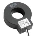
The E681x and E682x Series of current transducers provide a standard voltage output for use with data loggers, chart recorders, and power monitoring equipment. Both series have 0.333 V output. E682x devices are solid-core, while E681x CTs are split-core.
