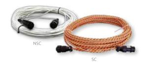
Sensing and non-sensing cables are designed for use with Zone and Distance Read panels. The sensing cables detect the presence of detectable liquid, and send a signal to the panel. The panel generates an alarm and pinpoints the location of the leak or spill along the cable's length. Sensing cables are designed for high accuracy and maximum reliability.
