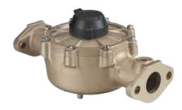
Nutating Disc positive displacement meters are a cost-effective solution for industrial flow monitoring. These devices are available in sizes from 1/2" to 2" and are capable of handling flows up to 170 gallons per minute. Maintenance is fast, easy, and rarely required. The meter houses a measurement chamber that contains a disc. Liquid flowing through the chamber causes this disc to nutate, or wobble. This motion is sensed by a magnet, which transmits flow data.
