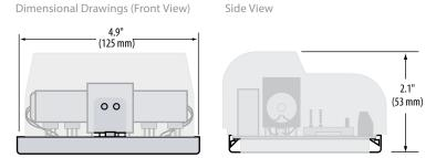
If the dust cover is ordered, the EP2 is mounted to a longer Snaptrack.
