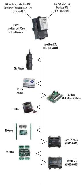
\*Supports SNMP only with a single E30A or E31A meter per E8951.
