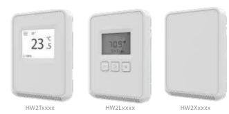
The HW2 Protocol Series of humidity sensors for living space is a flexible multisensor platform for use with BAS controllers designed to accept BACnet and Modbus outputs. HW2 Protocol Series sensors are available with three user interface options: touchscreen, LCD with three buttons and blank. Humidity and temperature sensors are included with all HW2 Protocol Series sensors.
