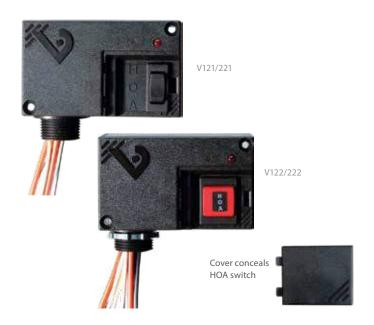
The Victory 121, 122, and 123 Series HOA relays have a concealed HOA switch for local control and troubleshooting with limited unauthorized switch manipulation. To further guard against control system override, the V122/V222 and V123/V223 are equipped with a monitored HOA. The V122/V222 provides a two-wire resistive output and the V123/V223 offers a three-wire digital monitor. Now you can enjoy the convenience of local control with none of the drawbacks.
