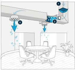
In-room ion density is dependent on a variety of factors, including proximity of the ionizing equipment to the occupied space, air flow rates and path of the ductwork within the building.
