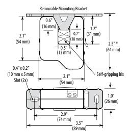
$<sup>^{\</sup>ast}$  Terminal block may extend up to 1/8" over the height dimensions shown.
