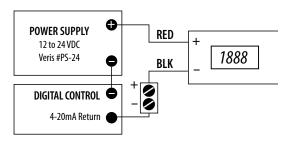
Wiring Diagram, 3-Wire, Sourcing Transmitter
