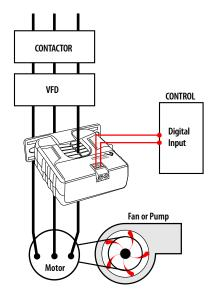
Note: The H904 is not intended for use in staged pump or variable inlet vane applications.
