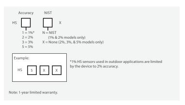
Generation 2 HS elements work with HW2 and CW2 sensor models.
