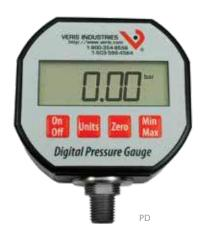
The versatile PD Digital Pressure Gauge can be used with any gas, liquid, or solid that is compatible with 17-4 stainless steel. The one-piece construction employs no silicone oil, welds, O-rings, or seals, making it the ideal universal pressure measurement device. The large LCD display shows the current reading, the selected scale, and the maximum and minimum pressure. All functions are easily controlled from the four panel push buttons located below the display.
