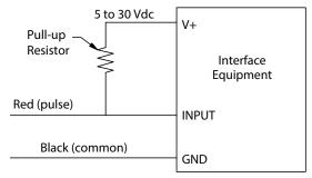
Note: Some interface devices may not have an internal pull-up resistor. Use a minimum 820  $\Omega$  resistor if necessary.
