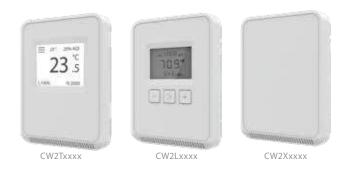
The CW2 Protocol Series of air quality sensors for living space is a flexible multi-sensor platform for use with BAS controllers designed to accept BACnet or Modbus outputs. CW2 Protocol Series sensors are available with three user interface options: touchscreen, LCD with three buttons and blank. CO<sub>3</sub> and temperature sensors are included with all CW2 Protocol Series air quality sensors. Models with VOC sensors and relative humidity sensors are also available.
