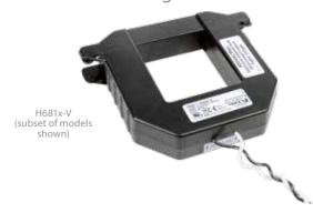
The H681x Series of 1 volt and 0.333 volt split-core current transformers (CTs) provide secondary AC voltage proportional to the primary (sensed) current. For use with power meters, data loggers, chart recorders, and other instruments, the H681x-V series CTs provide a cost-effective means to transform electrical service amperages to avoltage compatible with monitoring equipment.
