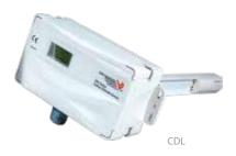
CDL carbon dioxide (CO<sub>2</sub>) sensors maximize energy savings, while helping optimize ventilation. These sensors allow ventilation systems to be controlled by the amount of CO<sub>2</sub> present in a space. The CDL Series detect fluctuations in CO<sub>2</sub> levels and signal ventilation systems to provide an inlet of fresh air optimal for the space at a given time saving energy and increasing tenant comfort.
