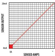
\*Adjusted with Span Potentiometer for Hx21 models; Factory-set per customer specification for Hx21SP models
