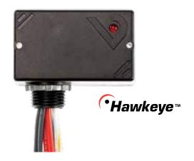
The H120 and H120NC offer a fixed current switch and SPST relay in a single externally mounted housing. Combining the current sensor and relay in one easy-to-install package eliminates the need to fit multiple devices into small electrical enclosures and simplifies the installation. Remove the labor associated with installing a separate current sensor.
