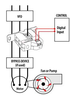
NOTE: The H614 is not intended for use in staged pump, variable inlet vane, and other applications in which the amperage changes under normal operation, independent of frequency. NOTE: (Optional) For added sensitivity in detecting amperage changes, use H614 devices on all three phases of the VFD
