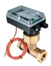
Series 380 BTU system provides a low-cost system for metering hot and cold systems. The 380 measures flow and temperature differential to accurately calculate energy. With BACnet, Modbus RS-485, or scaled pulse output, it can interface with many existing control systems.
