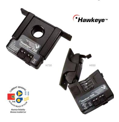
The Hawkeye Relay Combination Series combines an on/off status sensor and command relay in one package, saving the labor, wire runs, and space required to mount a separate relay. The switch and relay (not electrically connected) are in the same housing, saving space and cost. It is ideal for monitoring and controlling motors where belt loss is not a concern.
