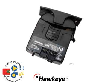
The Hawkeye 931 provides accurate load trending information with a proportional 4 to 20 mA output signal. These devices offer three amperage ranges for versatility, with easy slide-switch selection. The command relay is fully integrated in the device, but it is isolated from the current transducer. This combination makes these products ideal for start/stop control and status monitoring of motors, using one device instead of two.
