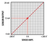
1. Field Adjustable from  $\pm 20$  A to  $\pm 200$  A (not applicable to customer-specified factory scaled models)
