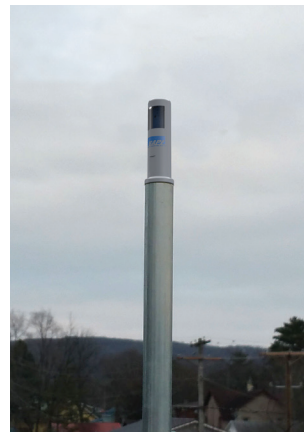
Light level sensor mounted in a parking lot facing north.
