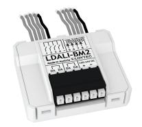
The LDALI-BM2 pushbutton coupler integrates up to four customary light push buttons and switches into a DALI channel. Alternatively, two of the four inputs can be used as analog inputs to connect devices like sliders, dials or even resistance based sensors like NTC temperature sensors.
