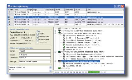
With a single mouse-click, the built-in report function creates reports (text files) showing the health condition of the investigated channel and gives hints and tips on how to solve problems on this channel.
