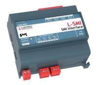
SMI is the acronym for Standard Motor Interface. SMI is a bus protocol used to control SMI sunblind motors for shading. Up to 16 motors can be connected to the bus. The L-SMI interface connects an SMI bus to a L-INX, L-ROC, L-GATE or L-DALI controller. Two SMI interface models are available.
