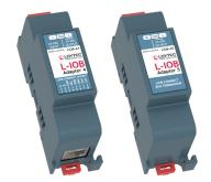
The LIOB-A2/A4 Adapters can be used to extend the LIOB-Connect bus and to connect an external power supply.
