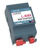
The KNX-Interface LKNX-300 allows the L-INX Automation Servers, the L-ROC Room Controllers, and the L-GATE Universal Gateways to interface to KNX devices connected to a KNX TP1 Bus. The LKNX-300 Interface needs to be connected to the EXT-Port on the L-INX/L-ROC/L-GATE devices.
