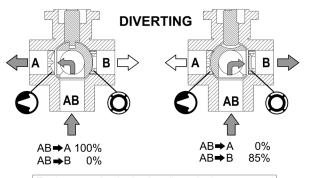
The A-port must be piped to the coil to maintain proper control
