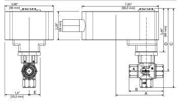
Actuator (V-FFV24) with 3-Way CVW
