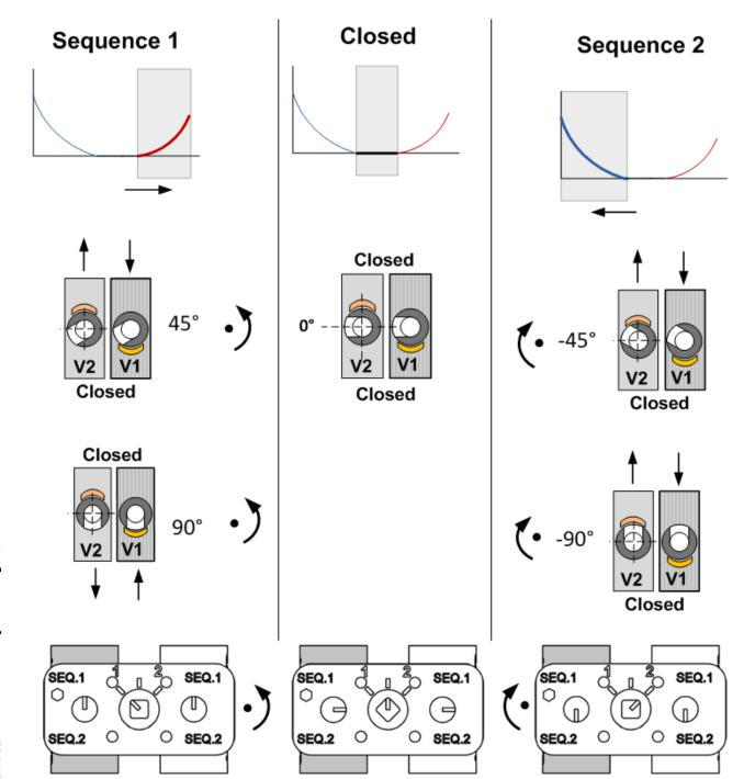
Both valves rotate in the same direction at the same time. Valve 1 (V1) has a disc oriented for CCW opening rotation. Valve 2 (V2) has a disc oriented for CW opening rotation. Each Cv has a Valve 1 and a Valve 2 version.
