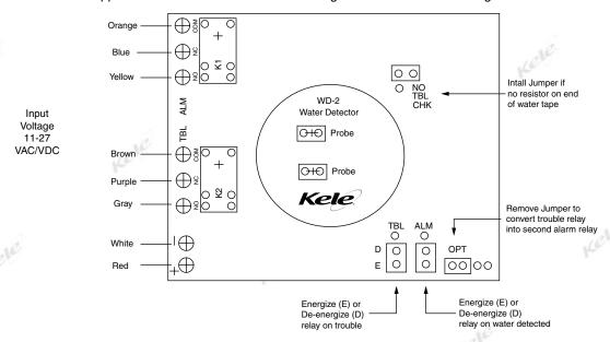
The Model WD-2-T tape includes a supervisory resistor mounted on the far end for the tape integrity self-check. A self-check disable jumper is provided inside for use with older or cut-down tapes that do not have the supervisory resistor.
