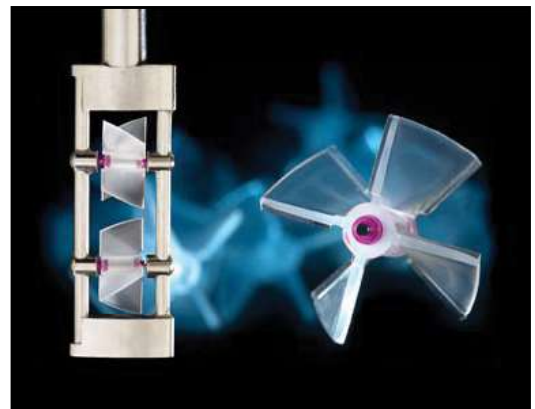
Axially mounted turbines riding on sapphire bearings virtually eliminate the mechanical load on the tungsten carbide shaft on which they ride.
