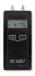
The Series 475 Intrinsically Safe Handheld Digital Manometer measures positive, negative, or differential pressures of air and natural gases in ranges from 1 in w.c. (0.249 kPa) to 150 psid (10.34 bar). The dual push pads on the front panel control the on/off, auto zero, and pressure unit selection, allowing for simple operation with no set up needed. When used with a Dwyer<sup>®</sup> Pitot tube (**0**), the Series 475 can also be used as an air velocity gage.
