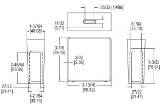
The **Model 480 Vaneometer**<sup>™</sup> **Swing Vane Anemometer** is a durable, economically priced instrument specifically designed to simplify the measurement of low air velocities. It is accurate to ±5% of full-scale to 100 FPM and ±10% from 100 FPM to the top of scale. It has a spirit level to ensure accurate readings and the large scales are easy to read and visible from both sides.
