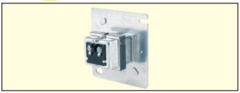
**UL** and **CSA** listed **Class 2 step down transformer** is mounted on a  $4\cdot1/4$  " square plate stand-off for direct installation in standard 4 " x 4" x  $1\cdot1/2$ " junction boxes. The A-699 is suitable for powering all Dwyer 4-wire transmitters and Model 660 Air Velocity Monitor.
