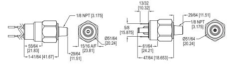
Designed for OEM applications, the Series A2 Subminiature Pressure Switch is economical and is equipped with high proof pressure capabilities for demanding applications. The A2 is available with either spade terminals or flying leads (submersible). Switches with spade terminals can be easily adjusted in the field.
