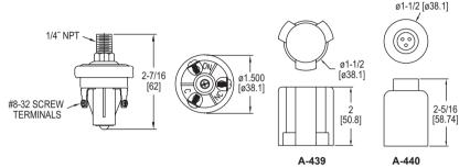
Series A6 Durable Pressure Switches have been specifically designed to stand up to extended duty applications. These switches are constructed with a polyimide film diaphragm and are compatible with a variety of fluids. For ease of installation, the switches come with a 1/4″ male NPT process connection and can be mounted in any orientation. The Series A6 pressure switches are compact and have great set point integrity, and feature simple, easy set point field adjustment.
