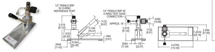
The **Series BCHP Low Pressure Calibration Pump** is able to generate pressure and vacuum for adjusting or calibrating pressure gages, transmitters, or switches. The pump is hand operated and has a pneumatic pressure range of -28 to 870 psi (-0.95 to 60 bar).
