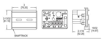
The **Model BPS-005 Low Cost DC Power Supply** is a regulated .5 A power supply that accepts 24 VAC input and provides an adjustable 1.5 to 29 VDC output. Output voltage adjustments are made using the on-board potentiometer while measuring the output with a multimeter. A compact snap track design allows the power supply to be surface mounted within a panel.
