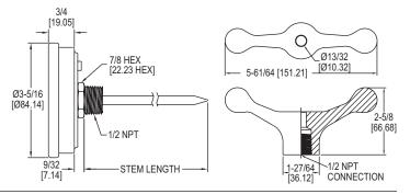
The Series BTLRN Long Reach Bimetal Thermometer reaches areas that other thermometers can't. A gripping handle is available as an accessory to comfortably hold the thermometer during temporary installations.
