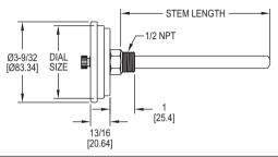
The **Series BTM3 Maximum/Minimum Bimetal Thermometer** accurately measures the current temperature along with a maximum read or minimum read temperatures.
