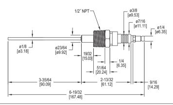
The **Model CLP Conductivity Level Probe** is used to determine the presence of a conductive liquid at a set level by sensing conductivity between the probe fitting and end. The Series CLP can be coupled with the Series TSWB Temperature Level Controller for a complete level control system.
