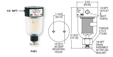
Model F222 & F451 Liquid/Particle Filters protect equipment and instrumentation from harmful contaminant's such as dirt, water and oil. Liquids are continuously coalesced and released through the manual drain valves. Replaceable filter element removes particles and droplets as small as 0.01 micron with 93% efficiency. Units have 1/4" female NPT inlet and outlet and manual drain valve.
