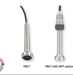
The Series FBLT Flush Tip Submersible Level Transmitters measure the height of liquid above the position in the tank referenced to atmospheric pressure. The transmitter consists of a piezoresistive sensing element, encased in a narrow 316 SS housing with PTFE coated flush diaphragm tip.
