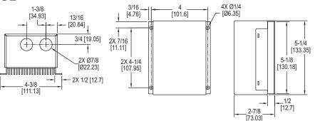
The Model FC-1000 Electronic Fan Speed Control provides precise speed modulation of small AC motors. Popular 0-10 VDC input works with most process controllers, eliminating the need for more expensive dampers, damper actuators, and linkages while improving overall energy efficiency of the system. This inexpensive unit enables variable control ventilation fans, condenser fans, and interfacing with VAV box controllers.
