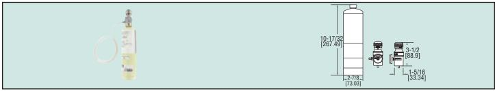
The Model GCK-200CO-2000CO2 Gas Calibration Kit provides a reliable flow of carbon monoxide and carbon dioxide to calibrate Dwyer® gas sensing transmitters. Every kit includes a span gas of 200 PPM carbon monoxide and 2000 PPM of carbon dioxide, a reference gas of 99.99% nitrogen, a 0.5 LPM flow regulator, and tubing. For convenient transportation, each kit is packaged in a hard carrying case. A certificate of analysis and material safety data sheets are included for both gas cylinders.
