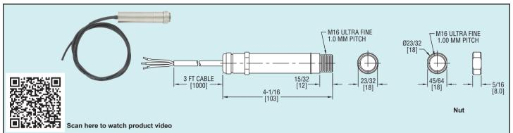
The Series ILA Non-Contact Sensors, measure temperatures from 32 to 932°F (0 to 500°C) and provide a linear 4 to 20 mA, 0 to 50 mV VDC or thermocouple output. The 2-wire signal is compatible with almost any indicator, controller, recorder, data logger, etc., without the need for special interfacing or signal conditioning. They are suitable for most materials such as food, paper, textiles, plastics, leather, tobacco, pharmaceuticals, chemicals, rubber, coal, and asphalt.
