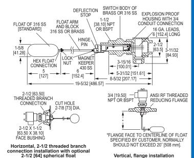
The Series L4 Flotect® Float Switch is a rugged and reliable float switch which operates automatically to indicate tank level
