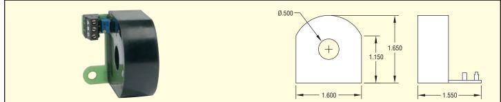
Love Controls Series LTTJ Current Transformers allow easy monitoring of the current flowing to your load. This easy to use device provides a 0 to 10 VDC signal into both low and high impedance circuits, and is easily scalable to your needs. Available in a number of different ranges, the Series LTTJ can be easily mounted on most Series LTP Solid State Relays for convenient wiring. Some models feature an LED for visual confirmation that current is flowing through the device.
