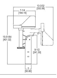
The **Series Mark II Wind Speed Indicator** indicates wind speed directly on the liquid filled scale reading in both miles per hour (0-80) and Beaufort scale (1-12). A metric model is also available, which reads the same as above, but reading 0-130 kilometers per hour. The Mark II Wind Speed Indicator is an accurate, economically priced option for measuring wind speed.
