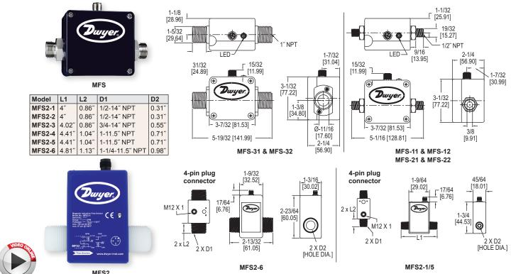
The Series MFS & MFS2 Magnetic Inductive Flow Sensors are compact, 316 SS body, in line flowmeters with pulse and optional analog 4-20 mA output. It is available in a variety of flow ranges from 0.25 to 52.8 GPM (1 to 200 LPM) and process connection sizes of 1/2" and 1" NPT.
