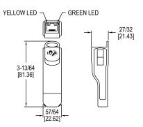
The Model MN-1 Mini-Node™ Communication Signal Converter is a low cost device that converts half duplex RS-485 serial communications signals into a signal that can be read by any computer with a USB port. The integral USB connector and RJ-45 connector reduces set up time by eliminating extra wiring. The Model MN-1 is powered via the USB connection which eliminates the need for an external power source. The compact size is great for field installation, control panels, and lab testing.
