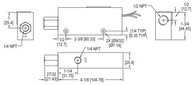
The **Series P1 Brass Flow Switch** utilizes a piston-type design for accurate detection of excessive or insufficient liquid flow rates. The switches have preset actuation points from 0.10 to 1.5 GPM for liquid flow.
