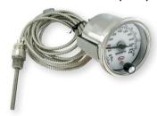
The Series RRT3 Remote Reading Thermometer with Switch combines an easy to read 3-1/4" dual scale dial thermometer and a SPDT relay. Color coordinated pointers display the current process temperature and set point.
