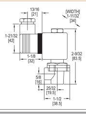
The **Series RSV Pilot Solenoid Valve** is used to operate the Series RDCV remote type diaphragm valve to air pulse clean filters in dust collectors. Consult factory for mounting of RSV valves with our DCT timer boards together in one enclosure all prewired.
