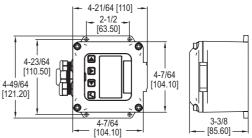
The **SERIES RTI2** Rate & Total Indicator is an indicator/transmitter that takes the pulse output signal from compatible flowmeters, displays flow rate and total, and provides output signals. It is compatible with the Series EFS2, IEFS, PDWS, and FLMG.
