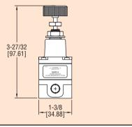
The Series SAFR is a miniature air pressure regulator that provides the highest level of regulation accuracy and repeatability available in a compact, lightweight body. This is ideal for applications that require exact pressure control and substantial flow capacity under variable operating conditions and limited space.
