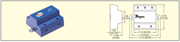
Model SSR-15 Intrinsically Safe Relay offers low power switching with solid state reliability and eliminates explosive conditions. Units are completely encapsulated and impervious to dust, moisture, or foreign material. Model SSR-15 can be mounted in any orientation and is shock and vibration resistant.
