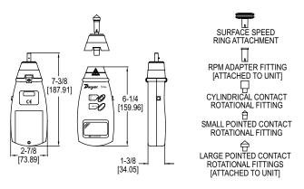
The Model TAC-L Portable Digital Tachometer measures rotational speed either by contacting a rotatable head to the shaft of the object or by using a photo sensor to detect the reflections from the laser. The housing is made of a strong, lightweight ABS plastic housing, which is designed to comfortably fit in the hand of the user. Supplied with this model are 3 contact rotational heads, a contact surface wheel, and a protective carrying case.
