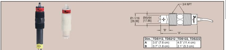
The Series TDS Thermal Dispersion Flow Switch offers solid state flow detection of non-coating liquids for pump and process protection. SPDT output allows for interfacing with remote PLC or relay control device. The adjustable switch point is factory calibrated at 0.2 fps with LED indication of flow and calibration status. Units feature selectable NO or NC operation and are not damaged by overranging flow velocities.
